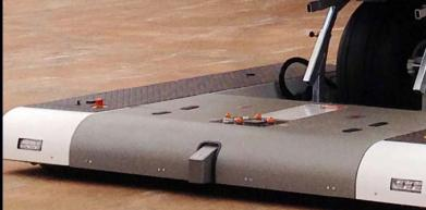
On production lines during aircraft manufacture, Mototok is a versatile tool that can be used with great flexibility. During assembly, Mototok automatically moves the aircraft fuselage to the individual assembly points. In very spacerestricted production environments, two synchronized Mototoks may also be used.
