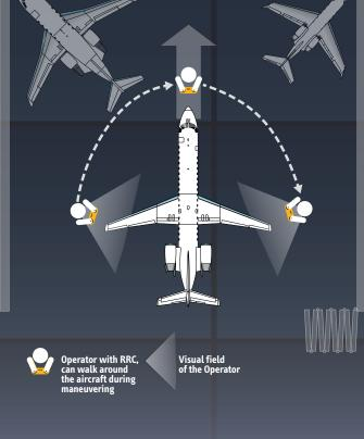
Circumferential view – only one person with a radio remote control (RRC) needed for moving the aircraft
