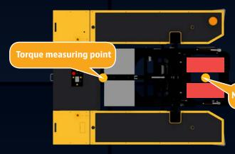
The forces and torques acting on the nose gear are measured by several weighing cells. Mototok's Intelligent Oversteering Protection System (I-OPS) prevents too high torques and initiates a counter steer action whilst either pulling or pushing the aircraft.
