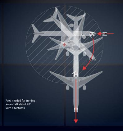
The nose landing gear is clamped on a rotating turntable to prevent damage to the nose wheel if the maximum turning angle of the nose wheel is reached. The aircraft tractor can continue to turn, but the turntable remains stationary.
